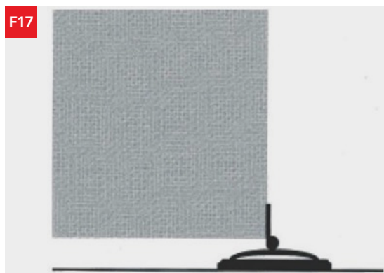
Figure 16: Type T1: Fixed seal on level floor
