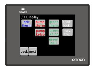
In the IO display users can view or control inputs and outputs for testing purposes when manual control is enabled it will stop any running process to avoid conflicts of operation and could allow one to test operation of components over riding all safety controls, as such this is password protected.
