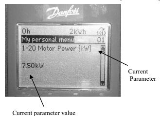
**My personal menu** These are the user modifiable parameters that are used when setting up the Aquaflow such things as motor power, pressure levels, automatic motor adaptation, motor ramp times, low and high-speed limits etc...
