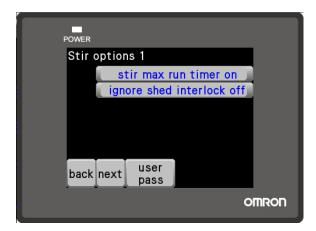
Above displays the feature settings you may tap on the button to turn the feature on or off as required, some settings are locked with a passcode so that only the installer or power user can alter them as they are set when the system is commissioned to suit the site.
