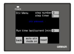
The example stir menu display as above shows the current step in the sequence (stem number) that indicates what part of the sequence the system in in which corresponds to the banner in the center of the display.
