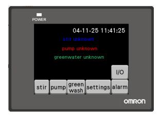
**The menu** display is used to control and monitor the system and to enable and disable features to suit the site requirements and features the user/ installer requires.
