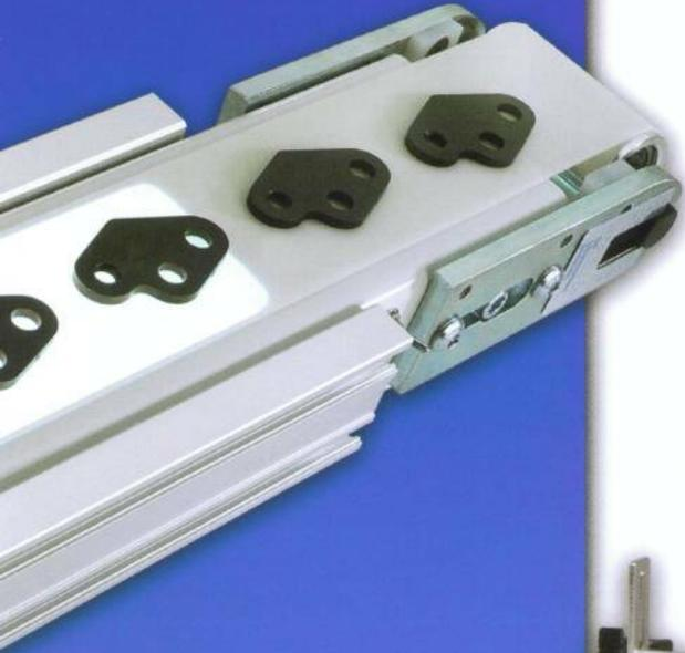
Accuvision projects a strong, uniform light field through the translucent belt of our low profile conveyor, illuminating part profile and appearance for automatic or manual vision inspection.
