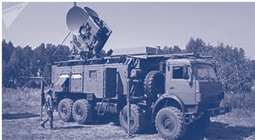
A Russian mobile electronic warfare system used to jam radar. Image credit: Sputnik News. 190
