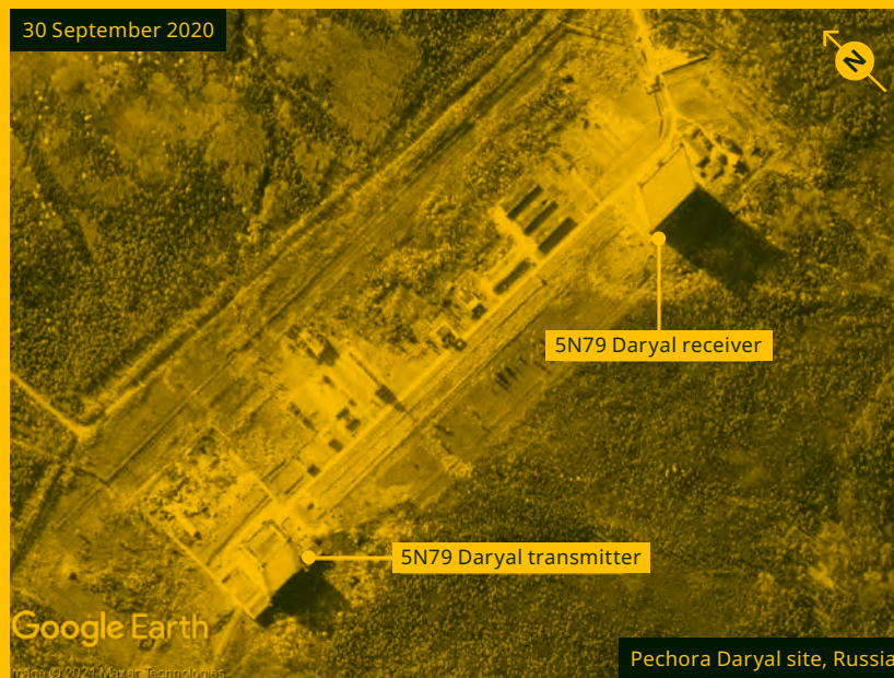
FIGURE 16-43 — DARYAL RADAR AT PECHORA
