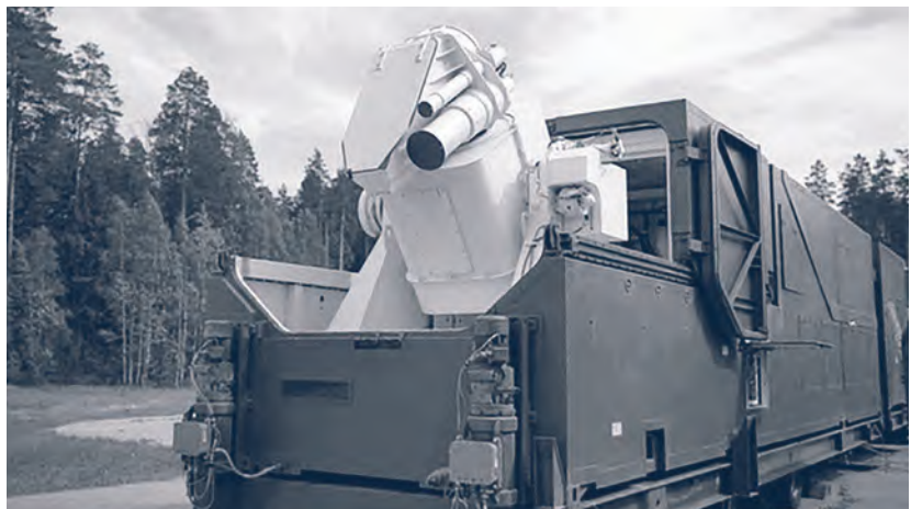
A Russian mobile laser system used to dazzle aerial and space reconnaissance assets. Image credit: Russian Ministry of Defense 307
