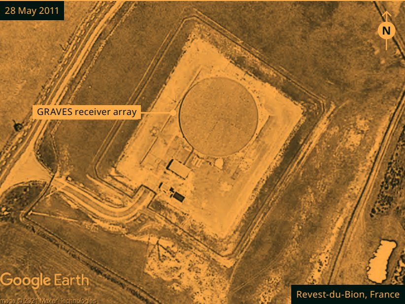
FIGURE 17-54 – GRAVES RADAR RECEIVER
