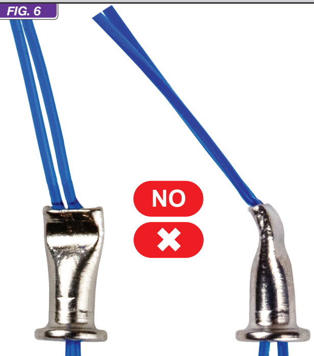
FIG. 6 For comparison, front and side enlarged views of an incorrectly crimped fastener that was not fully seated in the device tip
