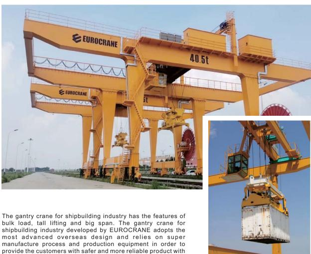
provide the customers with safer and more reliable product with more reasonable structure and more safety options, which will ensure the safety and service life of the crane. It has the following features:
