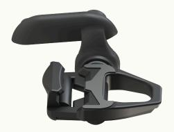
Similar to the handlebar and saddle sensors, the main purpose of the Body Rocket pedals are to measure aerodynamic drag. The assembly is straight forward - simply mount the pedals in the cranks arms, tightening to 30Nm. In order for the pedals to function you will also need to install a magnet which will be installed on the chainstay. After physically mounting the BR pedals
