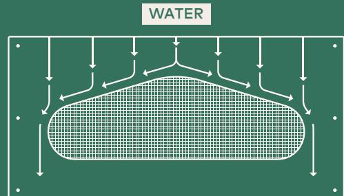
Unlike other products, this design forces water around the Primary Vent, preventing buildup and eliminating pooling behind it.
