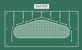
Unlike other products, this design forces water around the Primary Vent, preventing buildup and eliminating pooling behind it.
