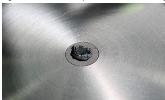
Figure 4.1: Binder sample on FTIR instrument crystal
