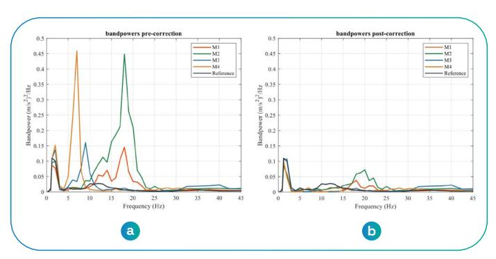
Figure 7: Bandpower of the signal from mounted smartphones - pre correction (a); post correction (b)
