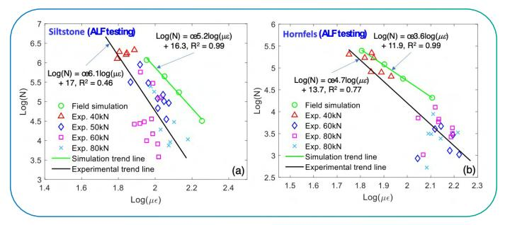
Figure 4: Comparison of initial micro-tensile strain versus fatigue lives (S-Nf curves) between field-scale simulation and ALF experiments for: (a) Siltstone materials; (b) Hornfels materials (Le et al., 2024).
