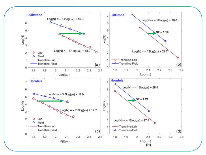
Figure 5: Shifting in strain and fatigue lives from lab to field scale: (a) Lab-to-field shifting for hornfels; (b) Lab-to-field SF for hornfels using SDE of 12 (Le et al., 2024).
