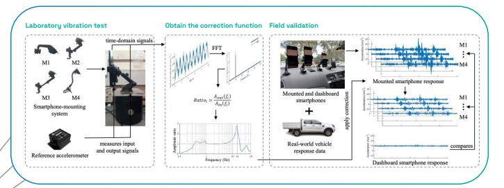
Figure 4: Schematic flowchart of the mounting correction method
