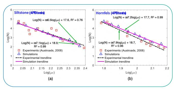
Figure 2: Comparison of initial micro-tensile tensile strain versus fatigue lives (S-N\_f curves) between simulation and experiments:
