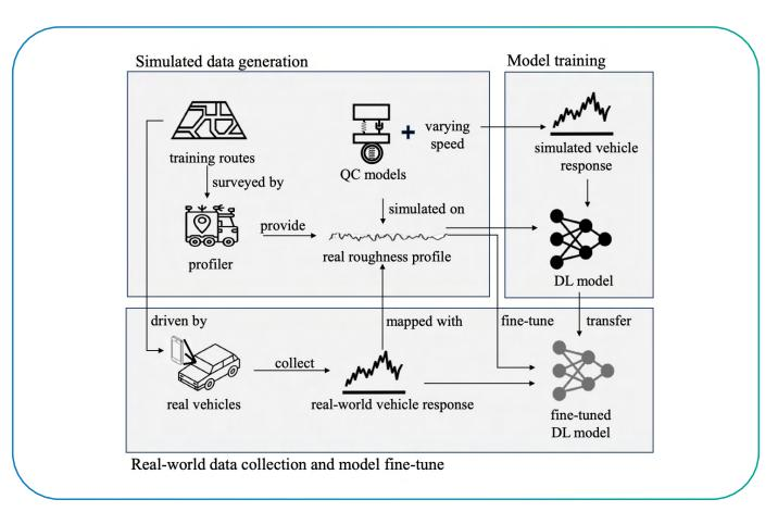
Figure 8 Schematic flowchart of the vehicle-based roughness profile estimation
