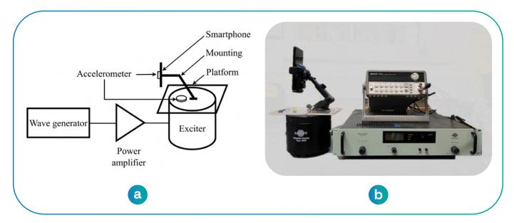
Figure 5: Schematic plot and Exciter set-up
