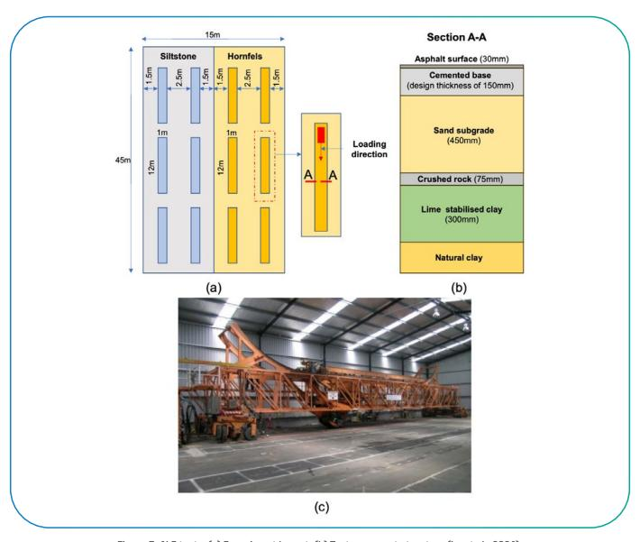
Figure 3: ALF tests: (a) Experiment layout; (b) Test pavement structure (Le et al., 2024); (c) The Australian ALF operating indoors at Dandenong, Victoria (Austroads, 2008b)
