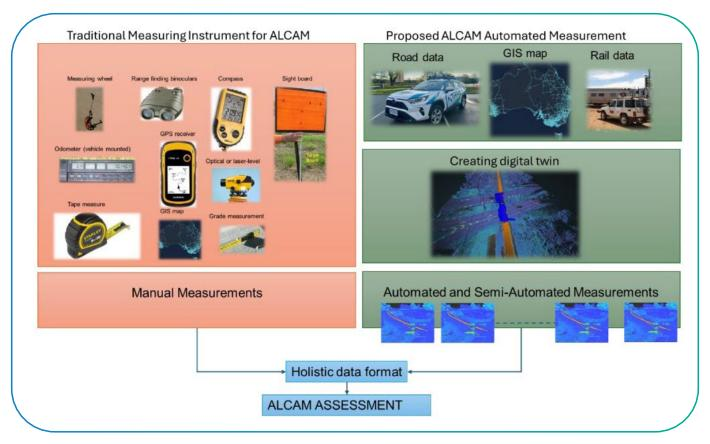
Figure 1: ALCAM Automation concept to streamline sight measurements for ALCAM surveys
