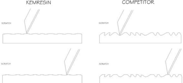
Other surfaces are more susceptible to scratches due to the contours of the surface catching sharp implements.
