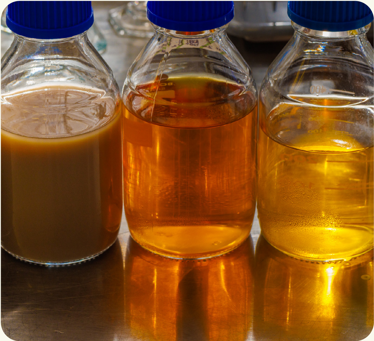
ABOVE Processing samples showing how Ceto-Boost™ changes the composition of the incoming digestate, eliminating organic solid material and releasing the inert, phosphorus-rich ash from the feedstock.
