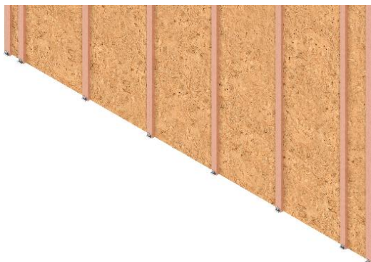
Row of clips between two boards on the substructure
