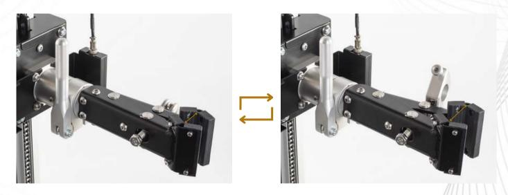
A spring between the clamp arms keeps the clamp open to the width you set it to, keeping the clamp arms from interfering with the seatpost during clamping and providing a firm feeling of engagement that a premium product like E-Billy requires.
