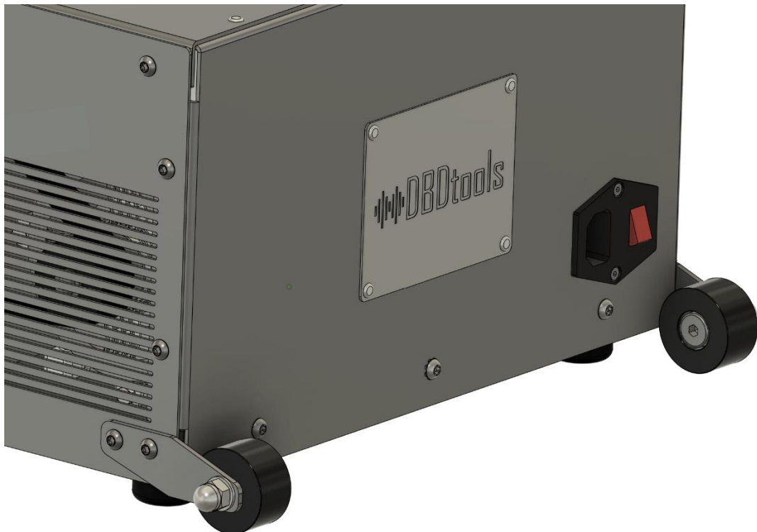
Figure 3: Install the Transport Wheels using a T25 key. Observe correct orientation - left and right wheels are different.
