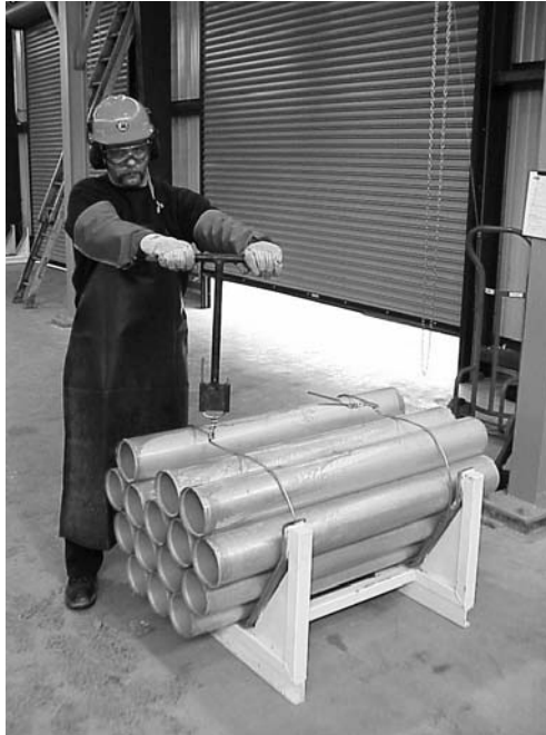
Figure 2 – Copper cathodes secured in the bundle. This bundle has 15 cathodes - the product from one 15 cell bank. The bundle is weighed and the weight used to determine current efficiency.
