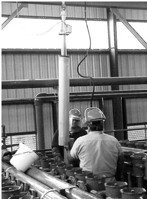
Figure 1 – Harvesting copper cathode from the plating cells. Copper cathode shown after removal of the split sleeve. The tops of cells with caps removed are visible. The operator in background is holding the split sleeve.
