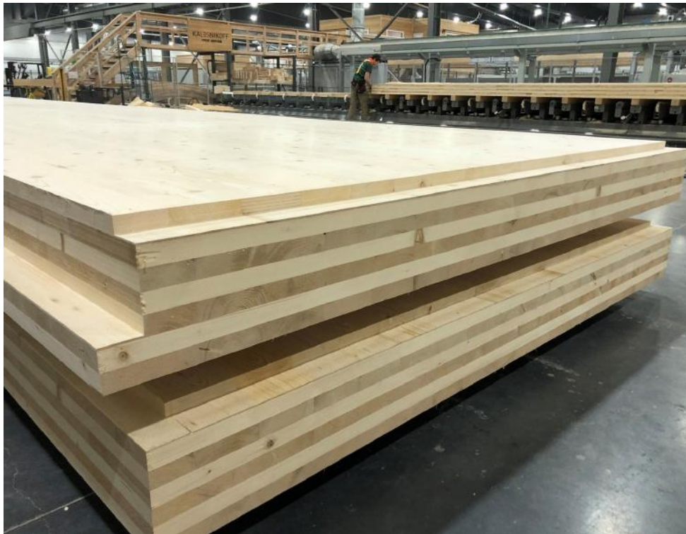
Photo of 7-ply CLT in Production. (Kalesnikoff)
