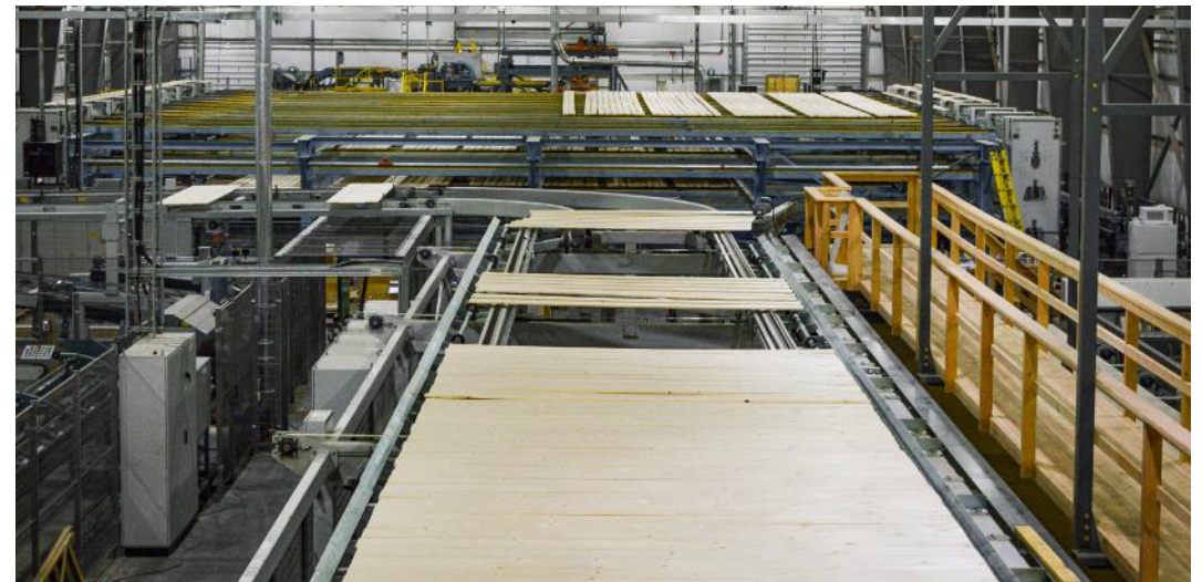
Photo of CLT Production (Kalesnikoff)
