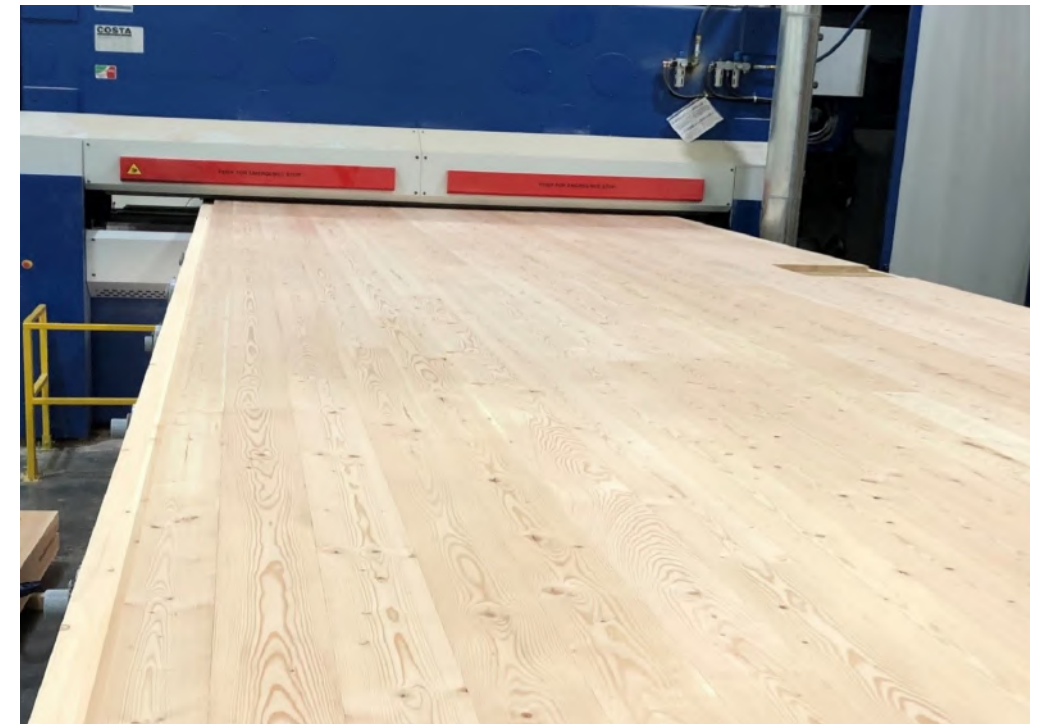
Photo of 7-ply CLT in Production. (Kalesnikoff)
