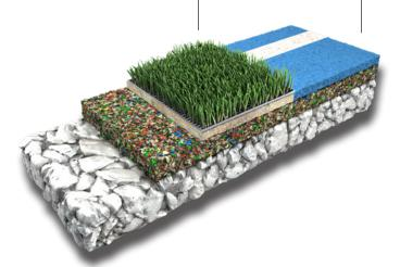
Melos EPDM Soft is the sustainable system component for the base layer of artificial turf pitches, athletics tracks, and multisport surfaces. Manufactured from high-quality virgin EPDM, the material is 100% REACH-compliant\* and meets the highest standards of quality and safety.
