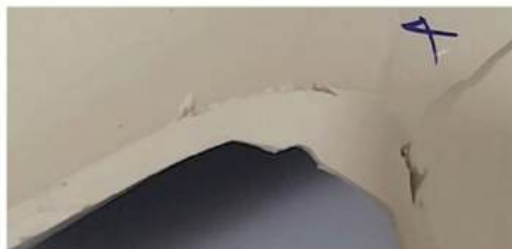
Figure 1 - No blistering or surface delamination observed after high temperature relief test.
