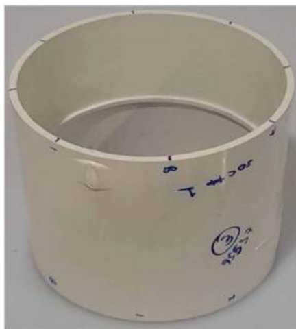
Figure 2 - DWV 100MM PLAIN STRAIGHT COUPLER as supplied
