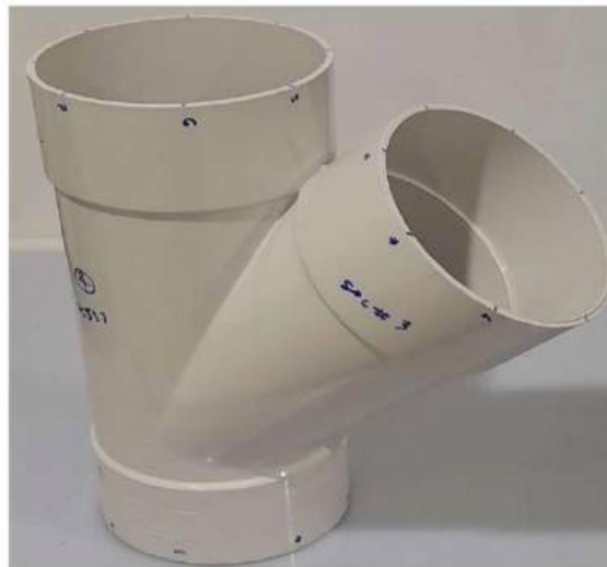
Figure 2 - 100mm x 45° - DWV Junction as supplied
