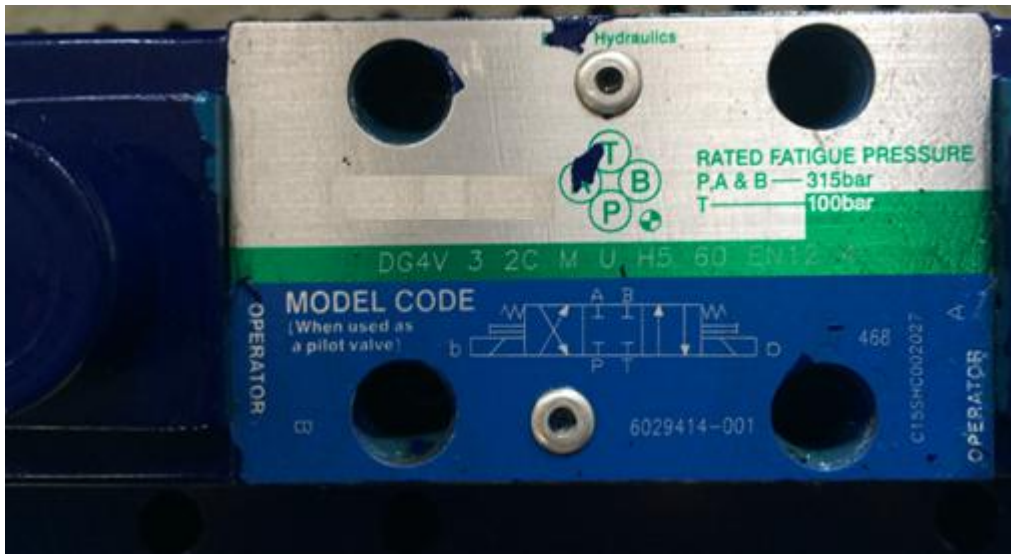
Schematic diagram of three-position four-way valve of core
