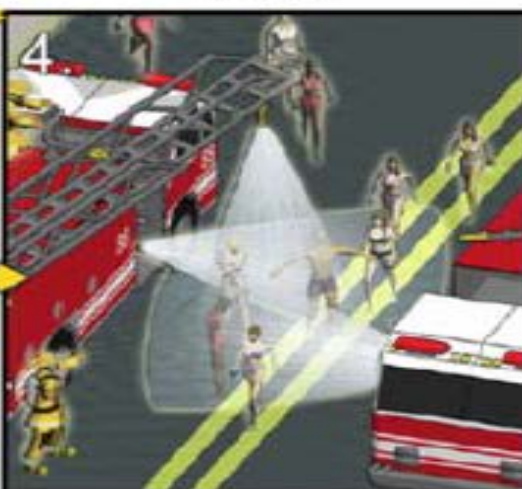
Apply continuous low pressure-high volume water deluge
