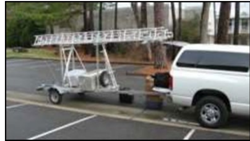
The HRMMST communications cache (12' Single Axle Trailer with a 65' Extendable Tower; Accompanying Tow Vehicle; Portable VHF Radios; Repeater; and Portable Marine Radios)
