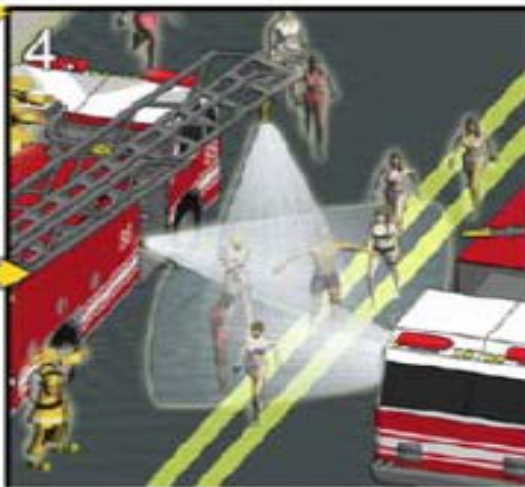
4. Apply continuous low pressure-high volume water deluge
