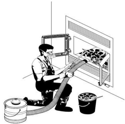
The chimney should be checked regularly for creosote build-up. Inspection and cleaning of the chimney can be facilitated by removing the baffle.
