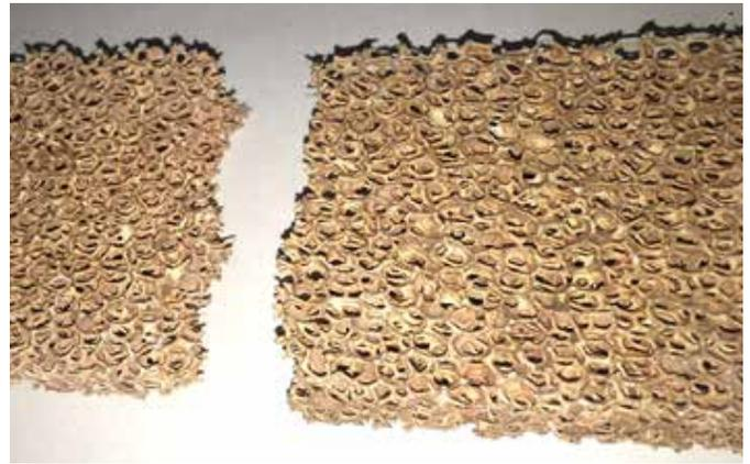
Combustor Problem - Broken Combustor
