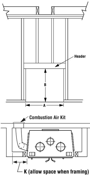
Combustible materials can NOT be used in the space directly above the fireplace. Do not fill the space above the fireplace with any material (Except the wood framing)
