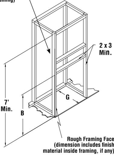
\*\* Total depth is 28-1/4" including the back standoff minus 1/2 inch for drywall to be flush with the facing.
