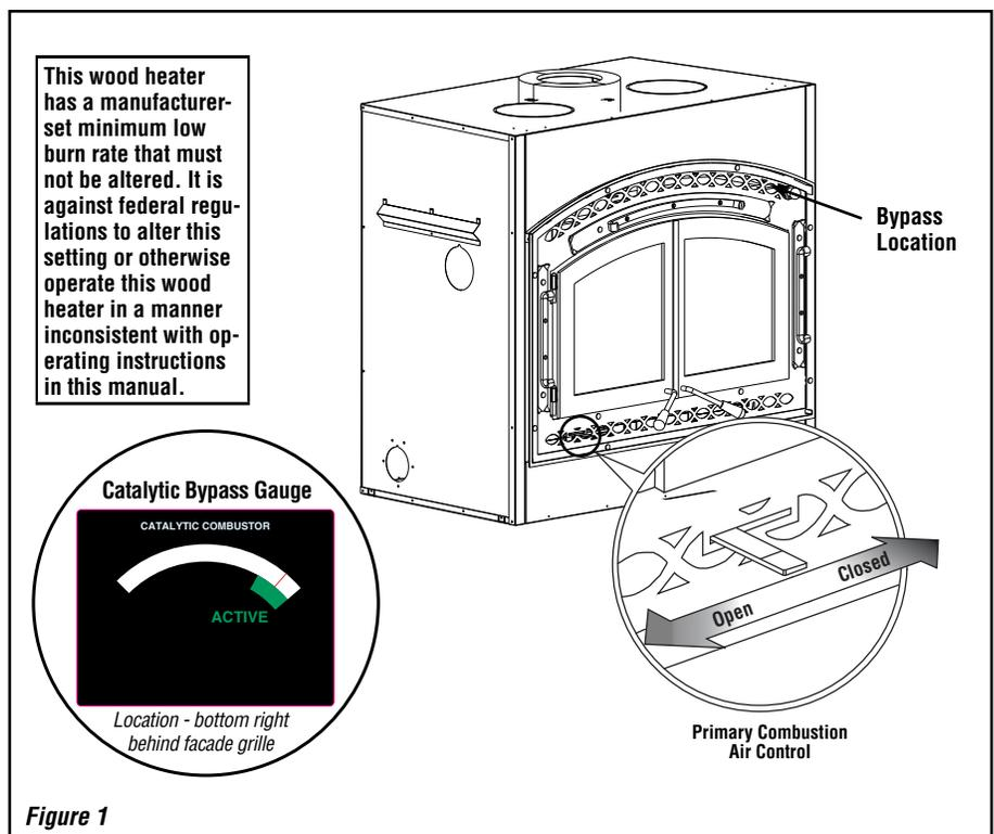
This manual describes the installation and operation of the IHP model Montecito Estate™ CAT catalytic equipped wood heater. This heater meets the 2020 U.S. Environmental Protection Agency's certified to comply with 2020 particulate emission standards using crib wood. Under specific test conditions this heater has been shown to deliver heat at rates ranging from 10,900 to 40,000 Btu/hr.
