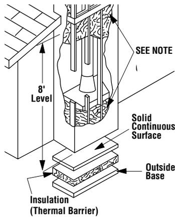
**NOTE:** It is recommended that the chase walls and floor be insulated in the same manner, using the same insulation, as the rest of the building, below the attic.
