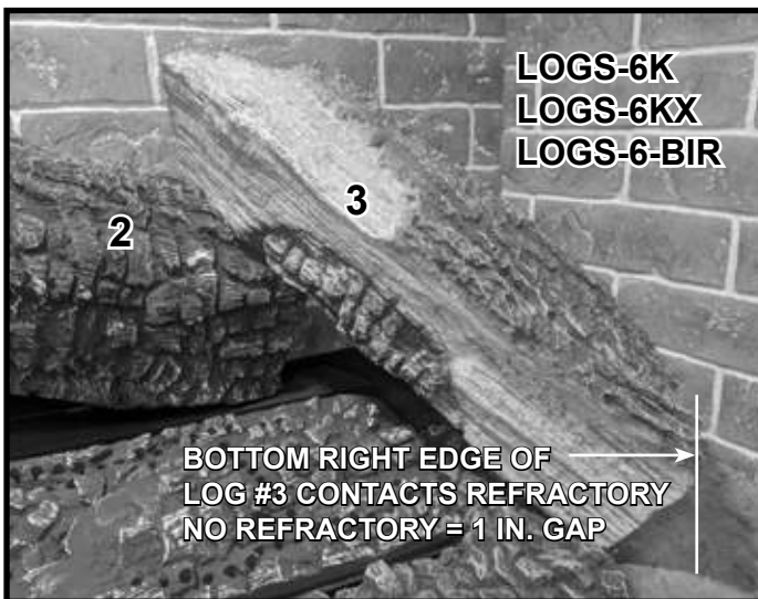
Figure 5.B Place Log #3 (LOGS-6K / LOGS-6KX / LOGS-6-BIR)
