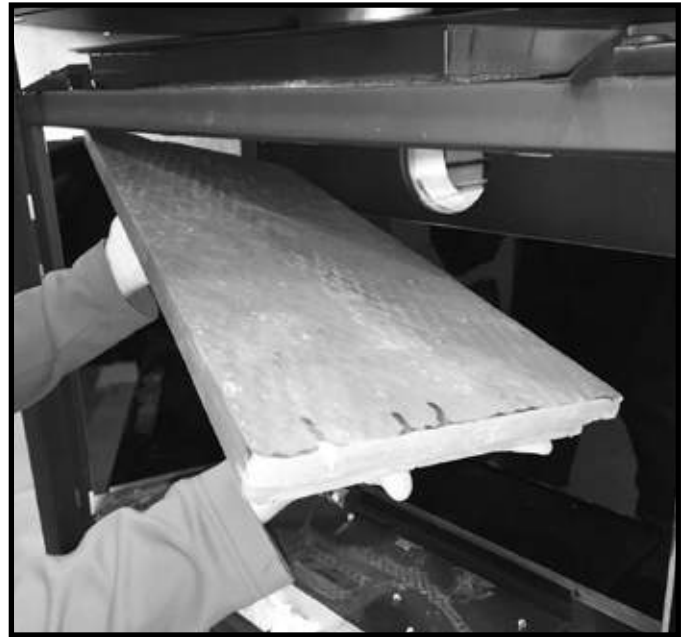
Figure 11.16 Install Top Refractory Panel
