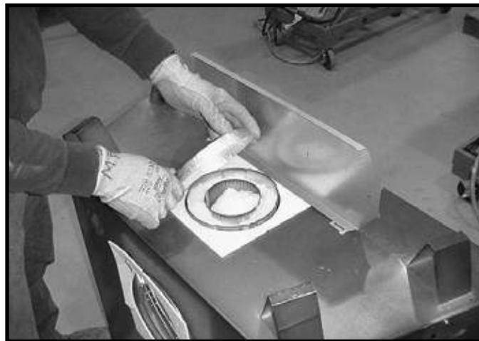
Figure 6.4 Remove the seal cap.
