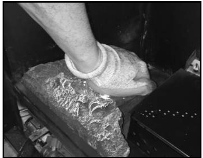
Figure 11.1 Press Left Hearth Firmly Into Place
