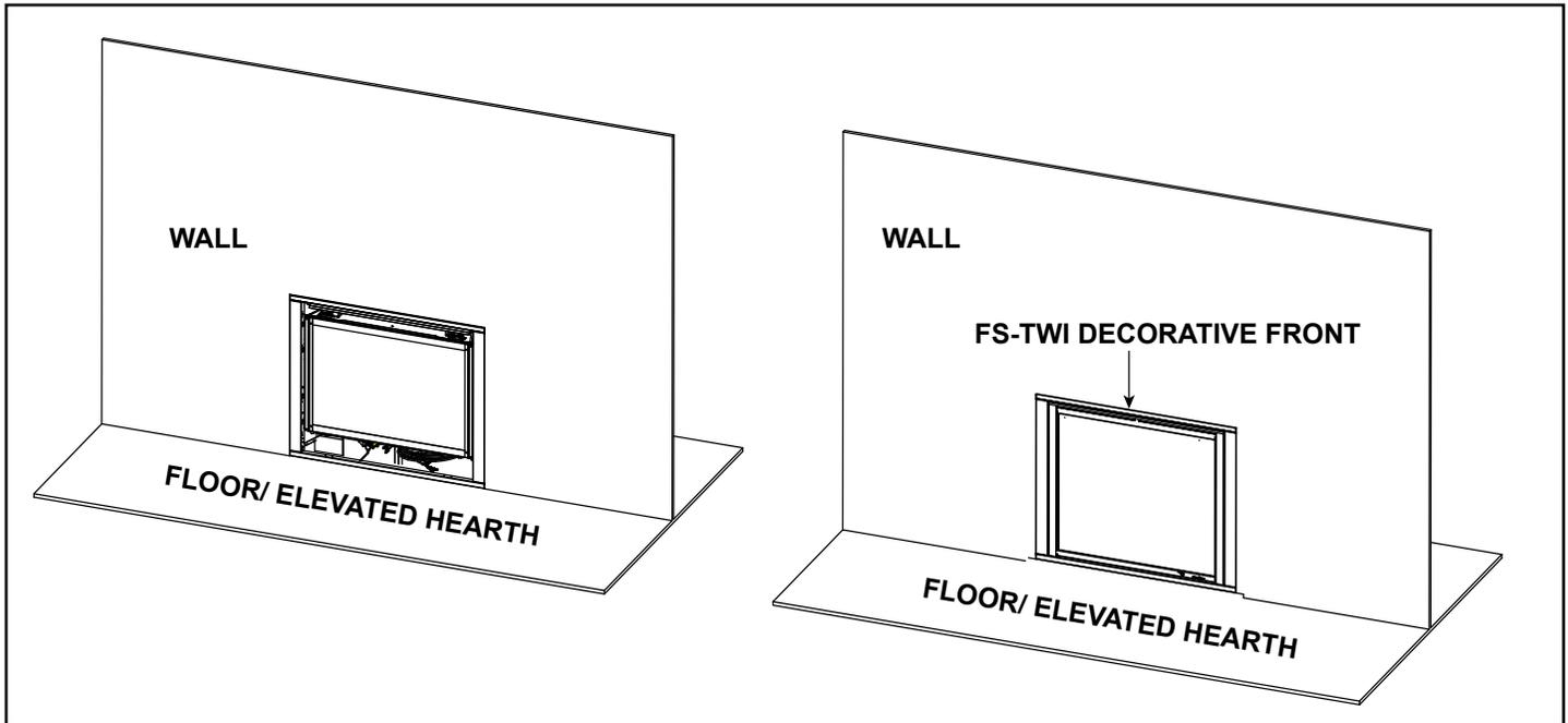
Figure 8.4 Appliance Installed on Floor or Elevated Hearth
