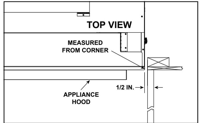
Figure 8.3 Clearances to Combustible Indoor Mantel or Mantel Leg
