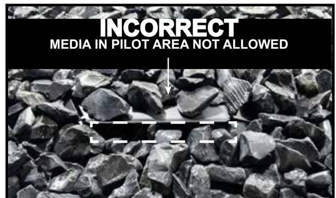
Figure 9.11 INCORRECT Media Placement
