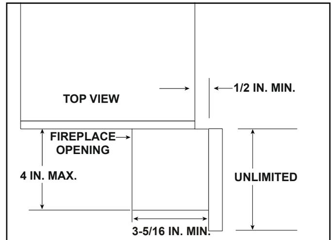
Figure 8.4 Clearances to Non-Combustible Indoor Mantel or Mantel Leg
