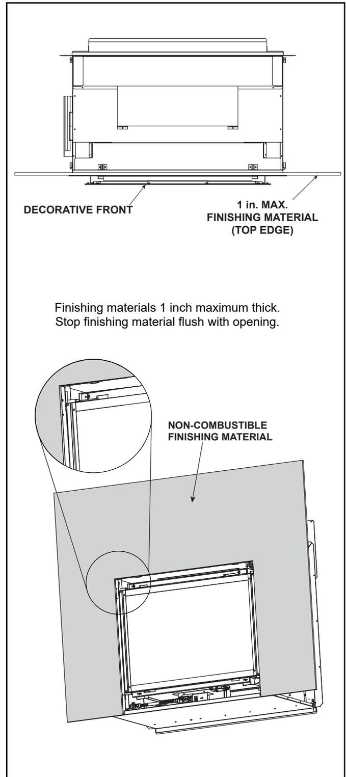
Figure 8.10 Finishing Material 1 Inch Thick or Less
