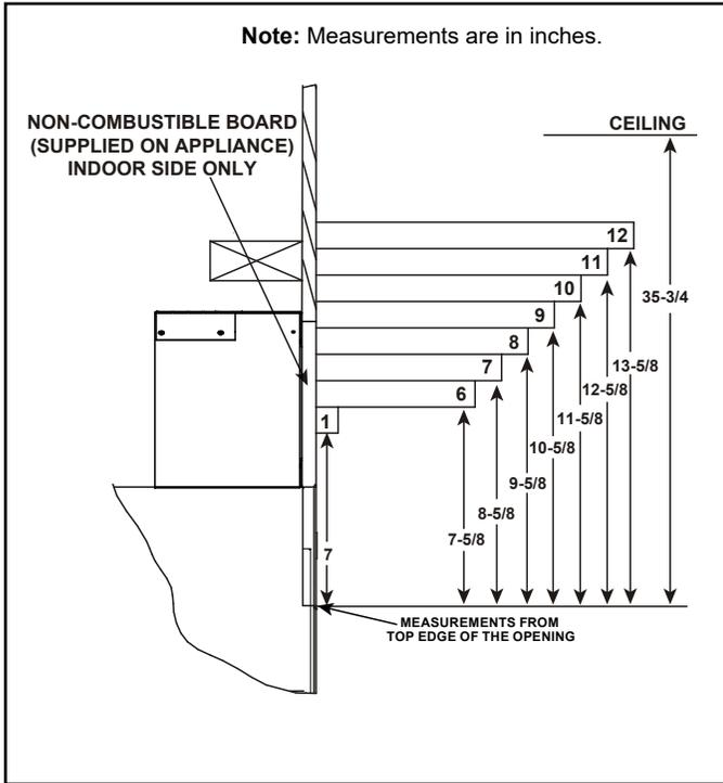
Figure 8.1 Clearances to Combustible Indoor Mantel
