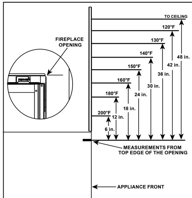
Figure 2.5 Maximum Interior Wall Surface Temperatures Above Appliance
