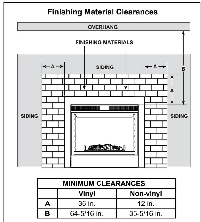
Figure 8.9 Exterior View - Finishing Material Clearances
