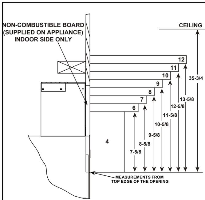
Figure 8.2 Clearances to Non-combustible Indoor Mantel
