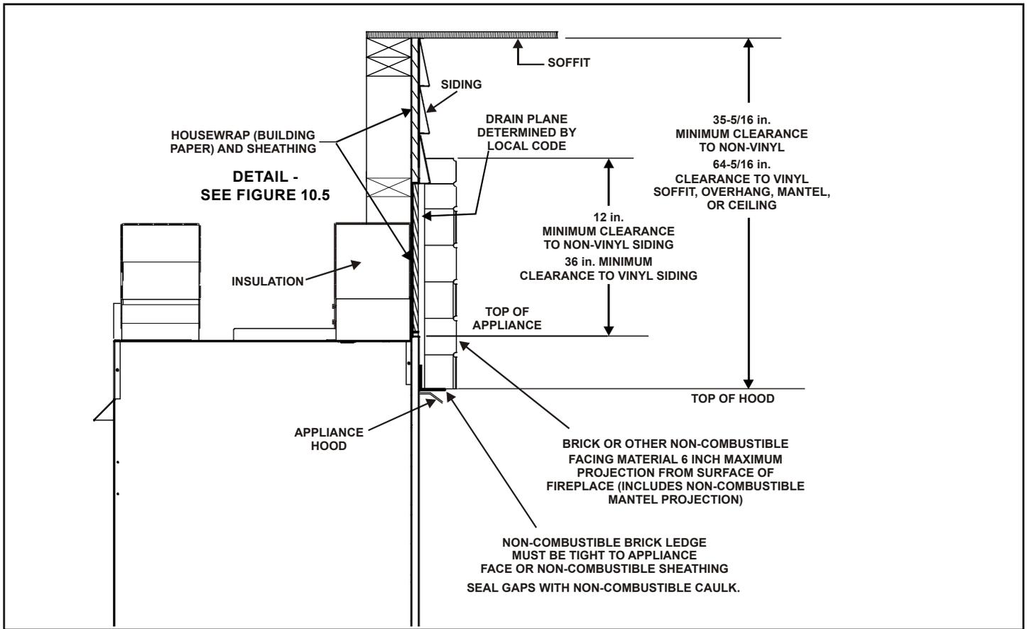
Figure 8.13 Exterior View with Non-combustible Facing Material
