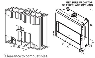
Dimensions above are in inches and millimeters. Product information is not complete and is subject to change without notice. Product installation must adhere strictly to instructions shipped with product. We recommend measuring individual units at installation. Assumes the use of 1/2-inch drywall. NOTE: Combustible material should not cover the face. Make sure you do NOT cover the decorative door opening.
