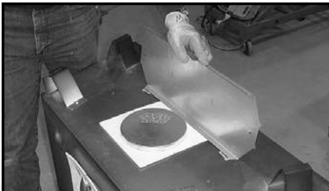
Figure 6.6 Rotate the top heat shield to the vertical position as shown above. The heat shield must remain in the vertical position.
