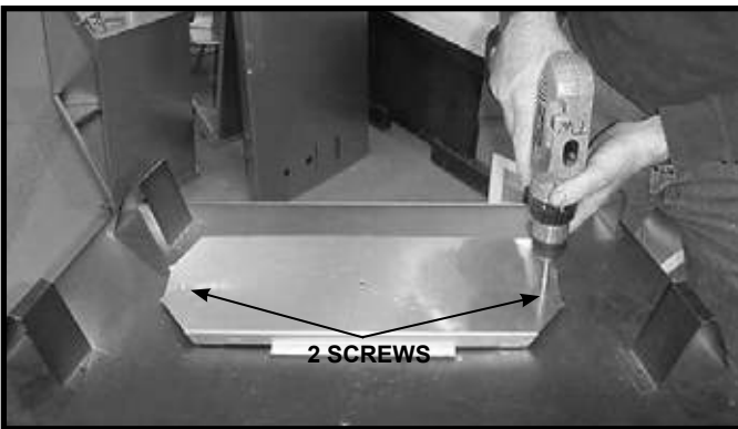
Figure 6.5 For top vent, remove the two screws holding the top heat shield in place. For rear vent, see Figures 6.12-6.16.
