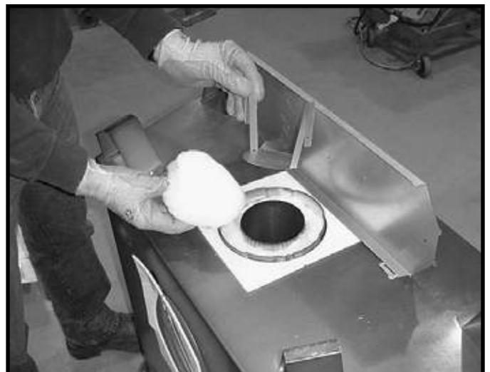
Figure 6.9 Remove the insulation basket and white insulation from the center vent pipe.
