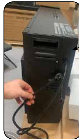
Wire Harness & Cover Plate Reinstalled.
