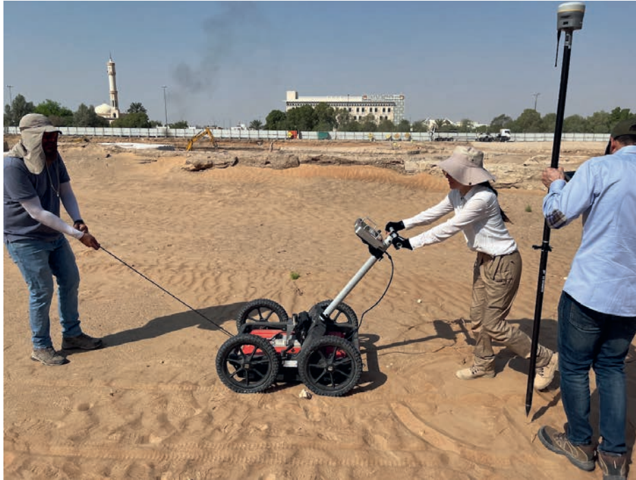
FIGURE 8. The team from the Earth Science Department of Khalifa University carrying out ground penetrating radar (GPR) survey in Area 3. The survey indicated the likely presence of more stone tombs in this area.
