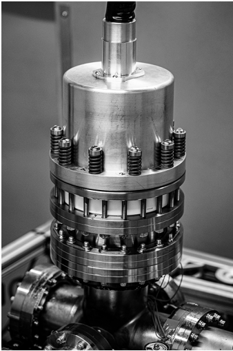
Figure 2 - Installation example of a Hammerhead feedthrough on vacuum chamber
