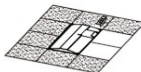
Step 3. Open the cover of junction box, Knock off the piece of side; Install serpentine coil in junction box.
