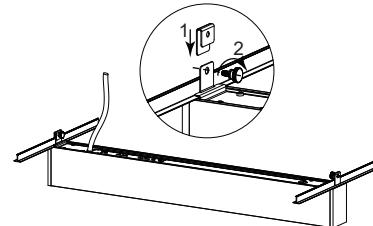
**STEP 1** Remove the plastic covers at both ends of the luminaire back.
