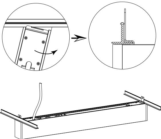
**STEP 7** Cover the gypsum board to complete the installation. (The gypsum board may need to have some edges and corners cut off to avoid power lines and installation brackets.)
