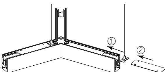
**STEP 6** Slide the connecting cover plate on the Y-shaped light fixture to the position between the two lights, covering their wire ports. Then, use the 4 screws from the accessory bag to secure the cover plate.
