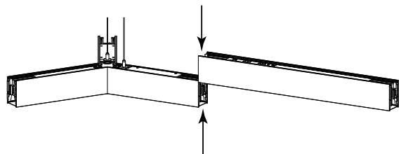
**STEP 2** Assemble the wire rope suspension kit and mount it to the ceiling.
