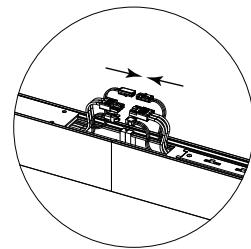
**STEP 3** Take out the Y-shaped (or V-shaped or L-shaped) connecting light fixture. Slide the suspension slider and the connecting cover plate into the back of the light body.
