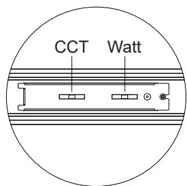
**STEP11** If you want certain light sections to remain off when powered: Set the power DIP switch on the back of those lights to "OFF". Make sure the switch for the sections you want to stay ON is closed at the corner connection on the light back. This ensures the best light beam effect.
