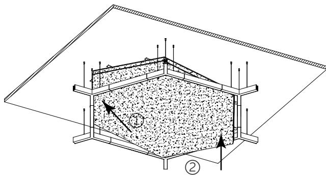
**STEP 2** Adjust the panel position so that the bracket extends beyond the panel and rests on the back of the light fixture. The panel is now installed.
