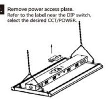
4. Power input from side: Remove knockout inendcap and install 1/2" " conduit, or B) install AC power cord with strain relief. Plug unused hole on power access plate with appropriate fitting
