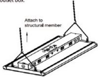
Power input from top: install 1/2" conduit or install AC power cord with strain relief into power access plate.
