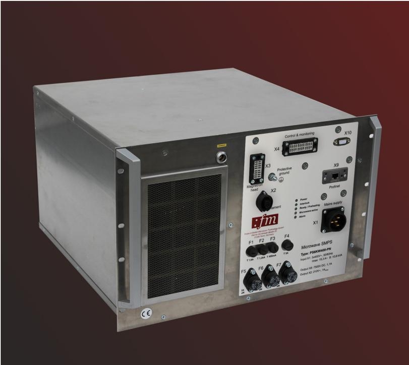
**FM - Low Ripple Switch Mode Power Supply for 5 kW Magnetrons @ 915 MHz** is a series of air-cooled power switch supplies. This model is able to power all 5 kW @ 915 MHz magnetrons on the market. Its output power can be regulated continuously between 600 - 6000 W by controlling through the PLC interface or fieldbus interface. The mains supply is available for 400, 440 and 575 V and working perfectly with FM-PS 5kW Magnetrons Microwave Head.
