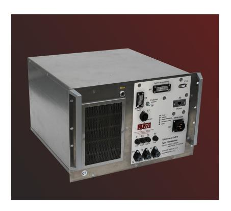
FM - Low Ripple Switch Mode Power Supply for 6 kW Magnetrons @ 2.45 GHz is a series of aircooled power switch supplies. This model is able to power all 6 kW @ 2.45 GHz magnetrons on the market. Its output power can be regulated continuously between 600 - 6000 W by controlling through the PLC interface or fieldbus interface. The mains supply is available for 400, 440 and 575 V and working perfectly with FM-PS 6kW Magnetrons Microwave Head.
