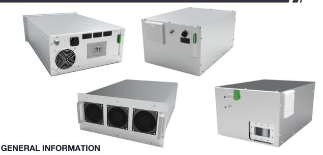
The BPAPFC-10 kW microwave generator is an air-cooled power supply for a 10 kW / 2.45 GHz magnetron. This power supply is designed based on modular interleaving technology to reduce input and output ripple as well as having the ability to protect the magnetron from over voltage and over current.
