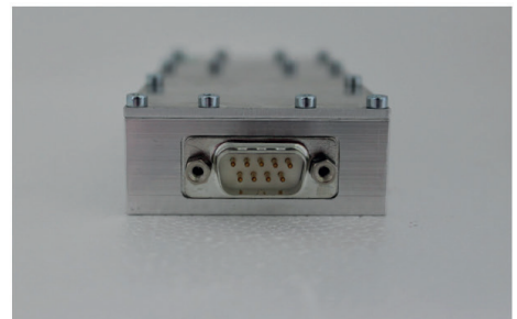
Back view PD1CH of the D-SUB 9-pin male Communication and DC connector
