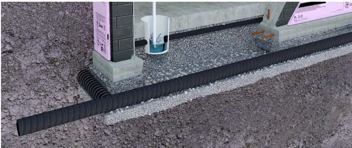
Cross section of a house foundation featuring black foundation drains.
