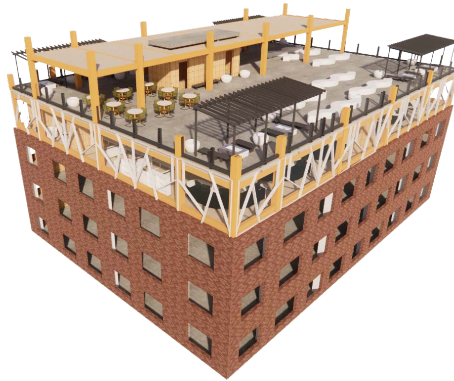
3-STOREY EXISTING STRUCTURE - SINGLE STOREY OPTOPPEN
