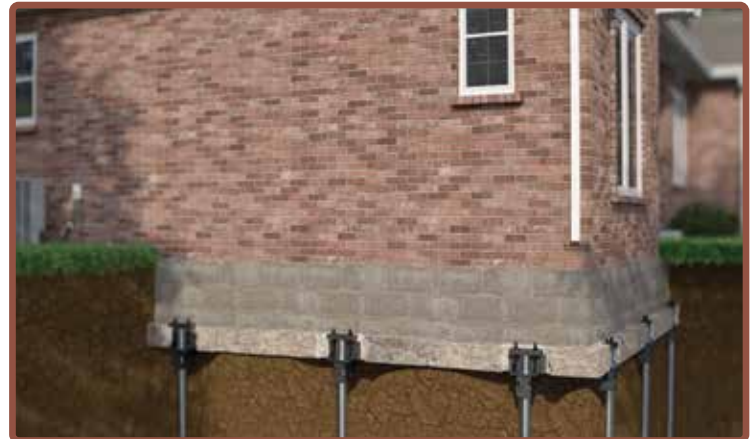
Installed piers are secure and undetected once the footer is covered.
