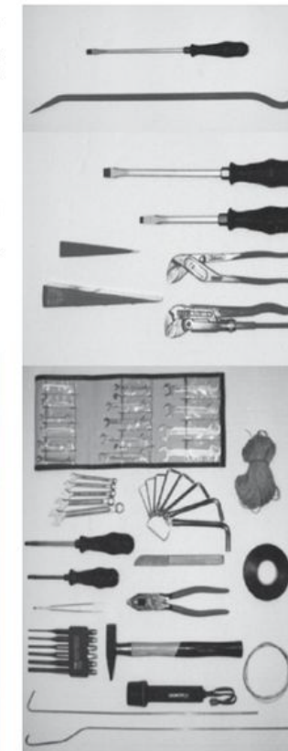
Tools used for testing 3rd security class doors.
