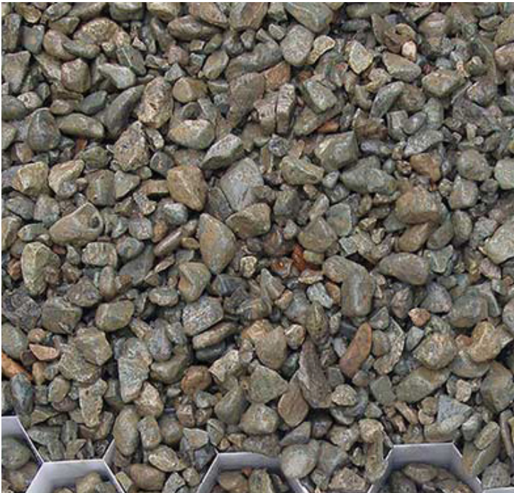
B Surface B - Reinforced gravel. 20mm river pebbles over subsurface stabilisation mat, or similar gravel access to private lots.
